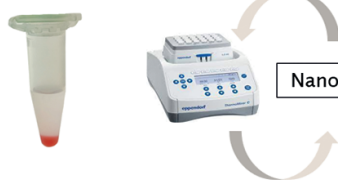
Figure 1: Workflow 1 describing the determination of mixing performance for all tested solutions using the workflow for the »Enzyme reaction« in Eppendorf Safe-Lock® Tubes 1.5 ml as an example. Step 1: The enzyme dummy containing Cochénille red and the reaction buffer were mixed by pipetting. Afterwards absorbance readings of the completely mixed solution were performed to determine the reference value. Step 2: The same reactants were mixed on the Eppendorf ThermoMixer C until the absorbance readings reached the reference value.
